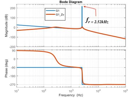
Fig. 2: Bode plot showing resonance damping by virtual impedance  $Z_v$ .
