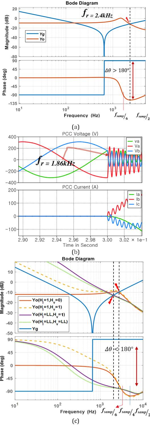
Fig.3: Bode plot showing the non passive region of the VSC (a), simulated result (b), passivity improvements steps (c).
