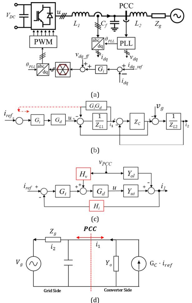
1: A generalized representation of a grid-connected converter system (a), the control block diagrams (b) & (c), and the closed-loop equivalent circuit.
