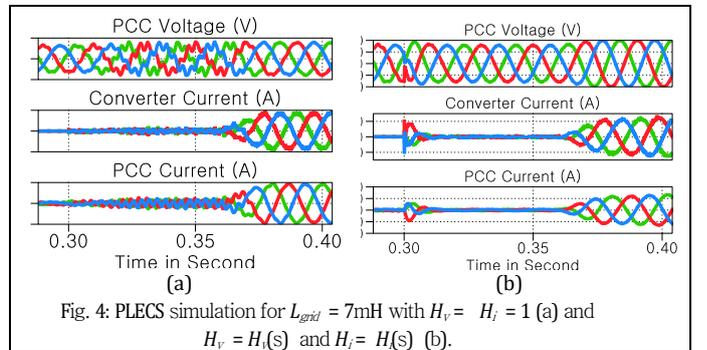
Fig. 4: PLECS simulation for  $L_{grid} = 7\text{mH}$  with  $H_v = H_i = 1$  (a) and  $H_v = H_i = LL$  (b).
