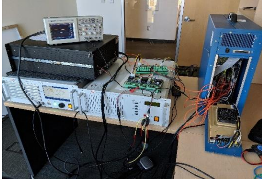
Fig. 5 Loopback testing using two power amplifiers
