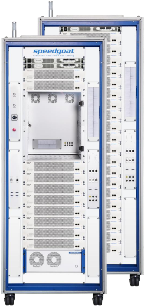
42U < 252 cells For 800 V battery packs testing designs
