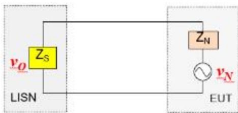
(a) CM 노이즈 전압측정 (a) The measurement of CM noise voltage
